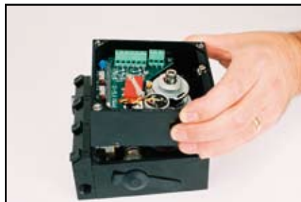
Place F5 unit on top, tighten screws
